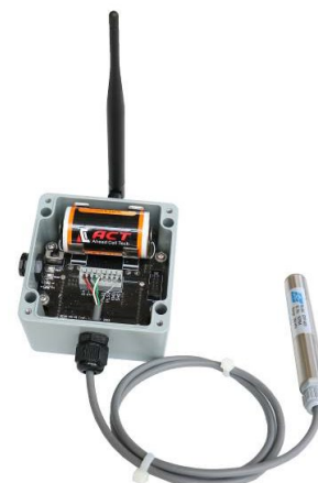
Vibrating wire piezometer connected to node
