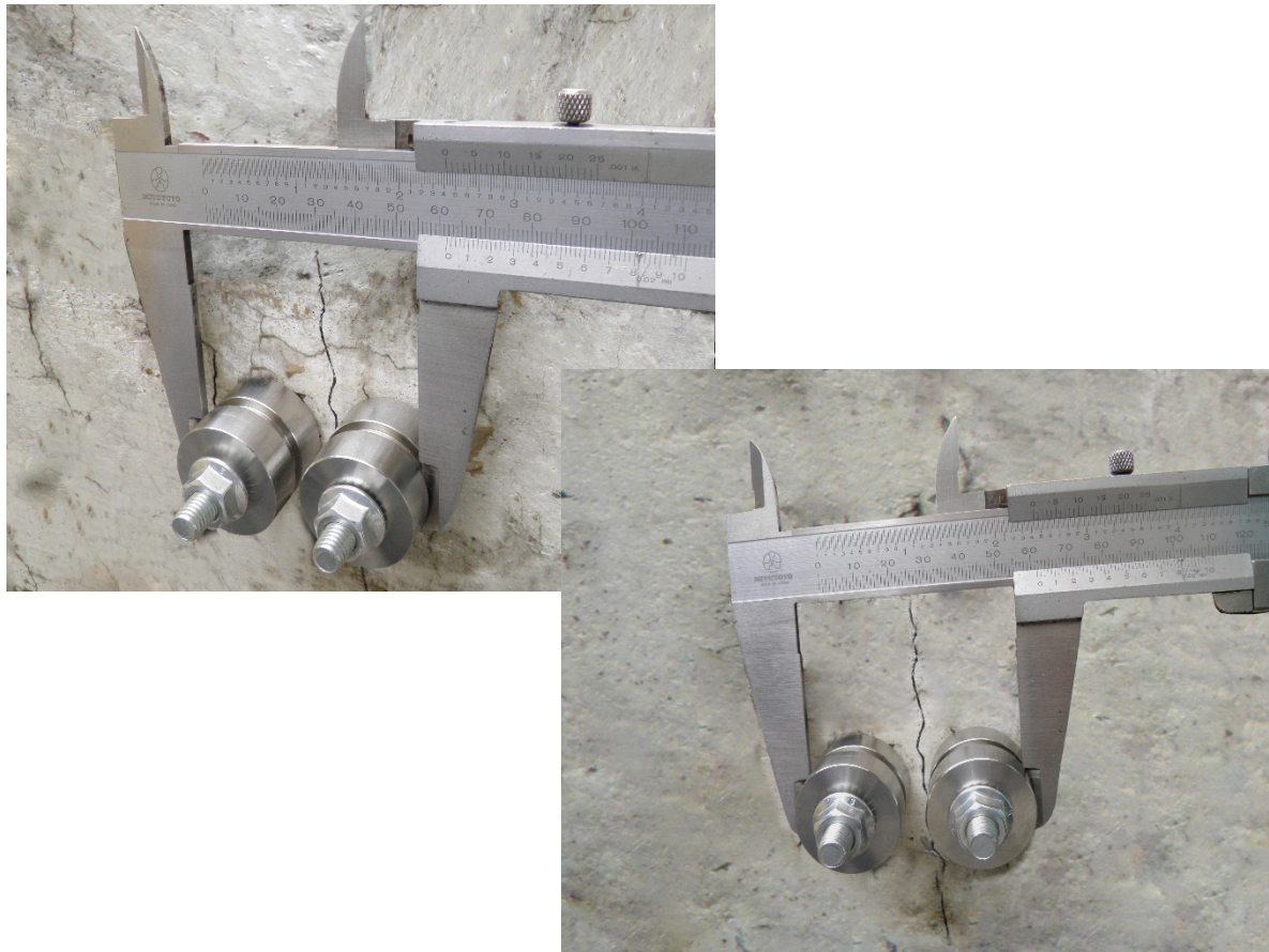
Figure 4: Taking readings of the datum/mounting blocks with Vernier Caliper
