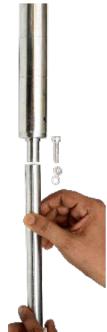
(b) Connecting the spacer tubing with the sensor
