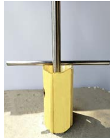
(a) Inserting retaining rod in the spacer tubing
