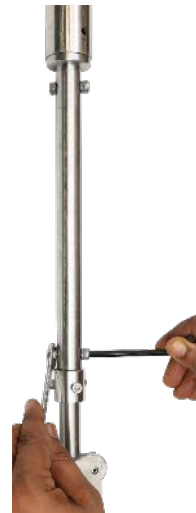
(c) Fixing sensor to gage coupler tubing
