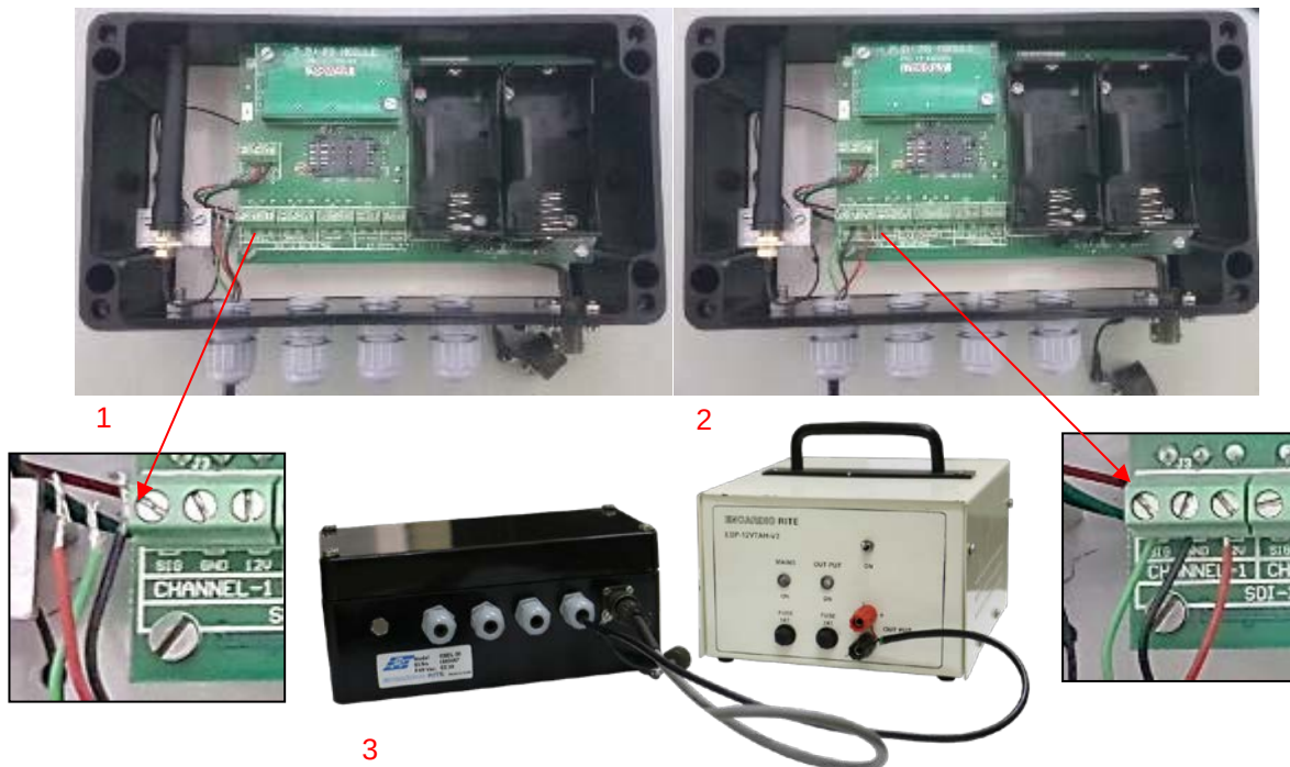
Figure 7-1 Connection of IPIS with ESDL-30 Datalogger:
