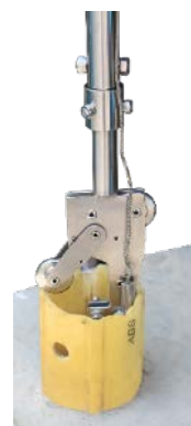
Figure 5-1 Installation steps for the IPIS sensors assembly
