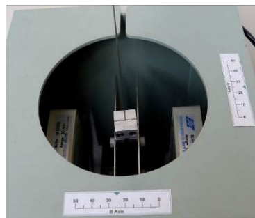
Picture 16 – Positioning scale for A and B axis
